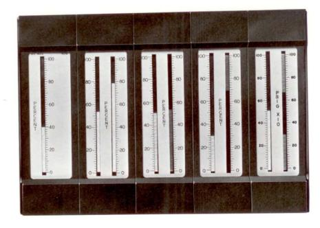
This 6-inch line-powered all-electronic instrument has a gas-discharge display comprising 203 closely spaced elements, each 0.150 inches wide. Measured variables appear as neon orange bars, alarm setpoints as bright red bars (flashing optional). Self-contained unit requires only signal and power input (120 VAC, 50/60Hz) for operation.
