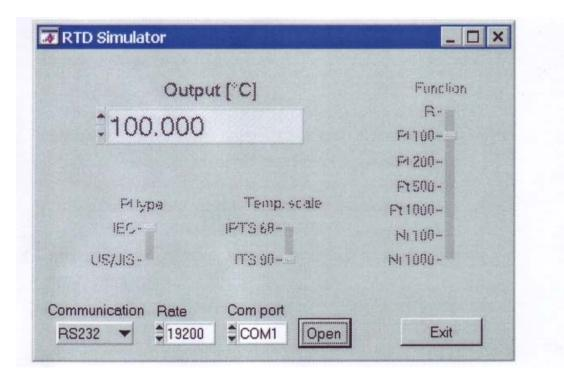
First use the Communication selection box to select the proper interface, in our case that is RS232. Then select the baud rate and communication port to use. After pushing the command button OPEN the program checks if the instrument is connected. If the instrument is found then it will be under computer control.
